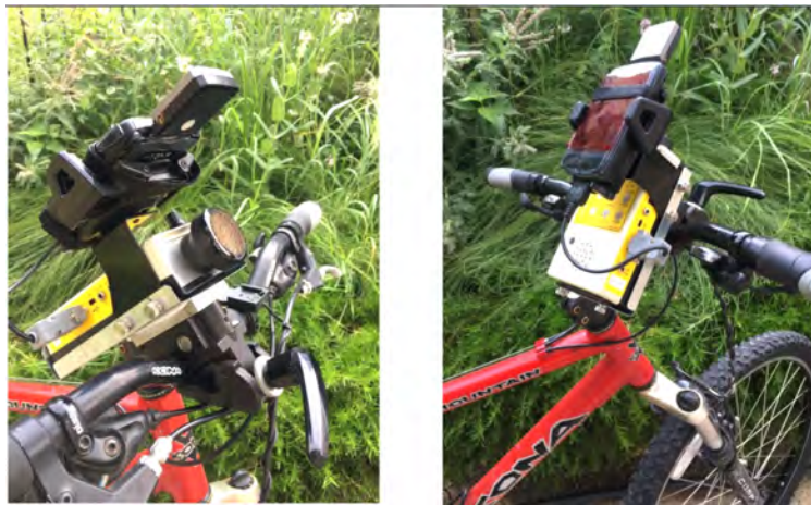
Figure 4. Housing and mount used to attach the bioacoustic monitoring equipment to a bike, kayak, canoe, or wheelchair.
